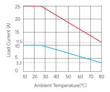
Note: the temperature of forced cool air cooling fin shall not exceed  $85^{\circ}\text{C}$
